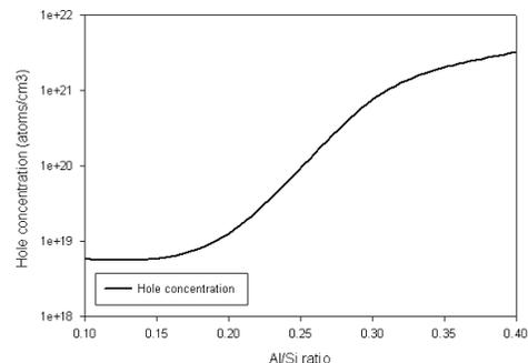
Fig. 2. Hole concentration of the Al-doped thin film Si on PET at different Al/Si ratios.
