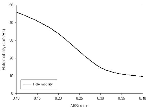
Fig. 3. Hole mobility of the Al-doped thin film Si on PET at different Al/Si ratios.
