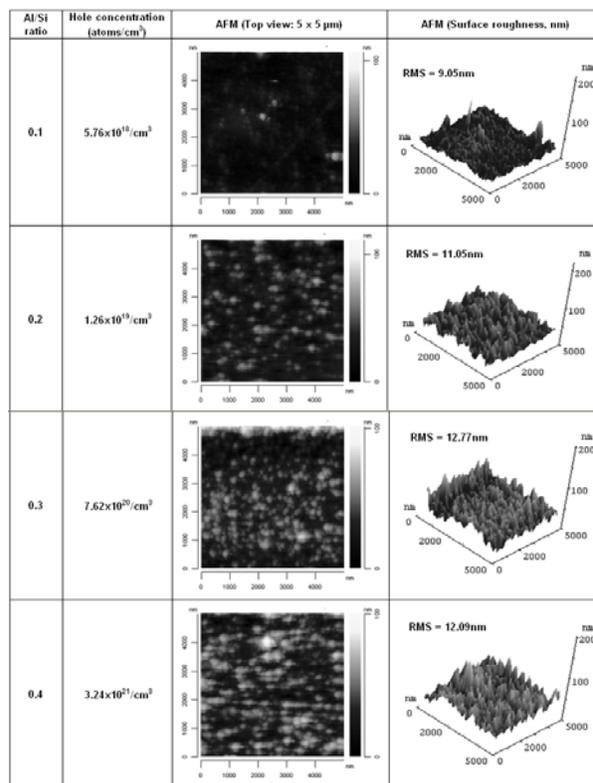
Fig. 4. AFM images ( $5 \times 5 \mu\text{m}$  spot size) of the Al-doped thin film Si on PET at different Al/Si ratios.
