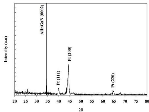
Fig. 2. The  $2\theta$  XRD spectrum of Pt Schottky contact on quaternary  $n\text{-Al}_x\text{In}_y\text{Ga}_{1-x-y}\text{N}$  thin film grown on sapphire substrate at annealing temperatures of  $400 \text{ }^\circ\text{C}$ .
