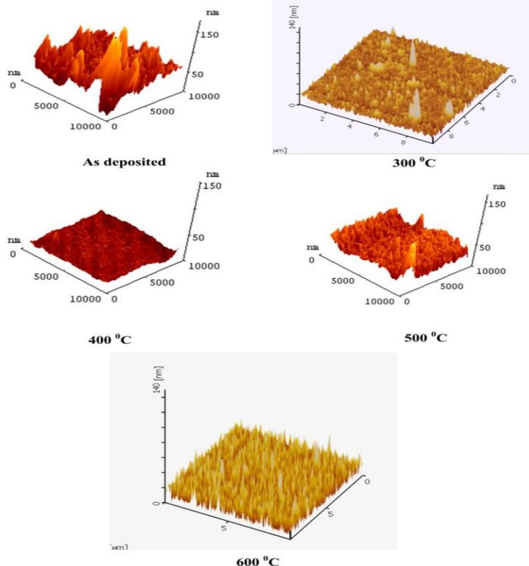
Fig. 3. AFM measurement of Pt Schottky contact on quaternary  $n\text{-Al}_{0.08}\text{In}_{0.08}\text{Ga}_{0.84}\text{N}$  film grown on sapphire substrate under different annealing temperatures.
