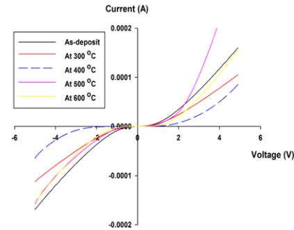
Fig. 4. I-V measurement of various annealing temperature of Pt Schottky contacts deposited on quaternary  $Al_{0.08}In_{0.08}Ga_{0.84}N$  thin film grown on sapphire substrate.
