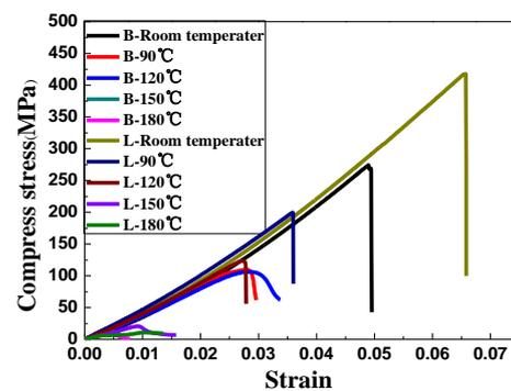
Fig. 2. The stress-strain curves for composites at 15 min of heating at different heating temperature.
