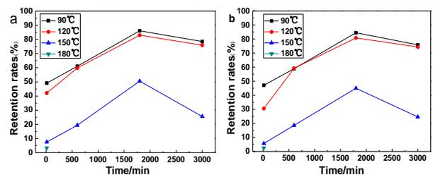
Fig. 3. The compression strength retention rate: (a) 3Dim-5Dir braid composites; and (b) laminated composites.
