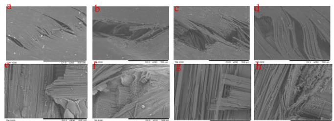
Fig. 7. The SEM photographs of 3Dim-5Dir braid composites and laminated composite fracture at 90°C with different heating time: (a, e) 90°C 15 min; (b, f) 90°C 600 min; (c, g) 90°C 1800 min; (d, h) 90°C 3000 min.
