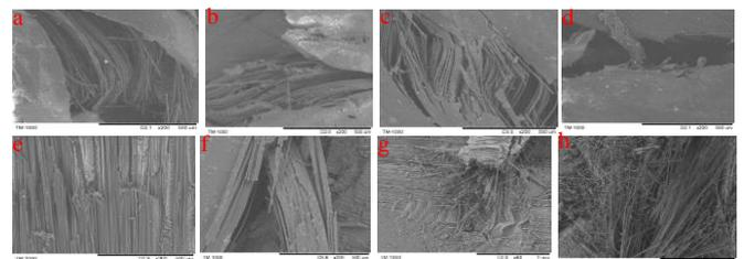
Fig. 11. The SEM photographs of 3Dim-5Dir braid composites and laminated composite fracture at 150°C with different heating time: (a, e) 150°C 15 min; (b, f) 150°C 600 min; (c, g) 150°C 1800 min; (d, h) 150°C 3000 min.
