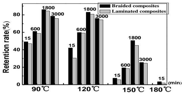
Fig. 4. Comparison of the compression strength retention rate at high temperature.
