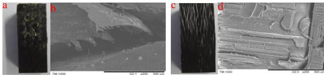
Fig. 12. The fracture photographs and the SEM photographs of compression specimen at 180 °C (a) the fracture photographs of 3Dim-5Dir braid composites; (b) the SEM photographs of 3Dim-5Dir braid composites; (c) the fracture photographs of laminated composites; and (d) the SEM photographs of laminated composites.
