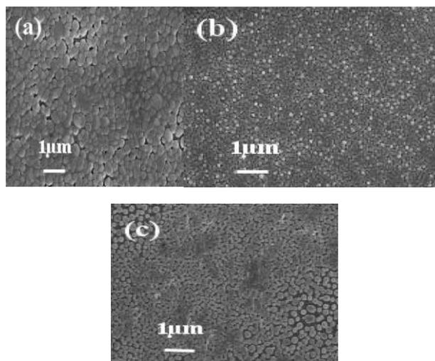
Fig. 2. Surface morphologies of the films on different substrate materials: (a) the glass film; (b) the quartz film; (c) the mica film
