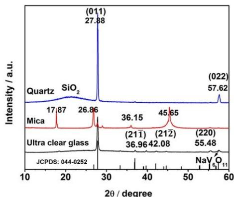
Fig. 1. XRD patterns of the films on different substrate materials
