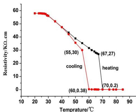
Fig. 3. Resistivity-temperature relationship of VO<sub>2</sub>(M) film prepared on the silicate glass
