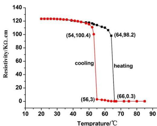
Fig. 5. Resistivity-temperature relationship of VO<sub>2</sub>(M) film prepared on the mica substrate
