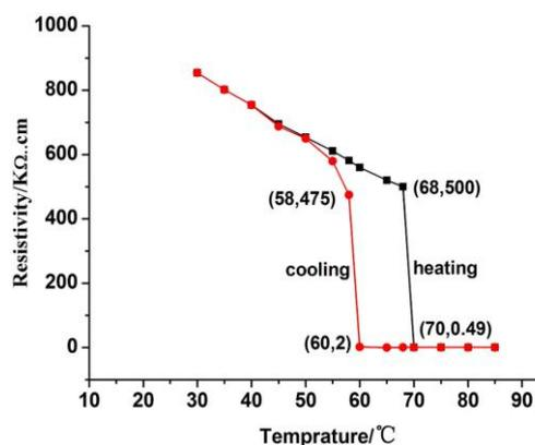
Fig. 4. Resistivity-temperature relationship of VO<sub>2</sub>(M) film prepared on the quartz substrate
