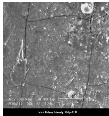
Fig. 6. Surface machined without of Al 2 O 3 powder.
