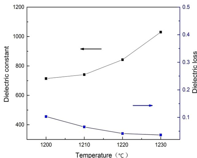
Fig. 4. Dielectric constant and dielectric loss as functions of different crystallization temperatures (measured at 1 kHz)
