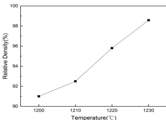
Fig. 1. The variation curve of relative density of samples with crystallization temperature
