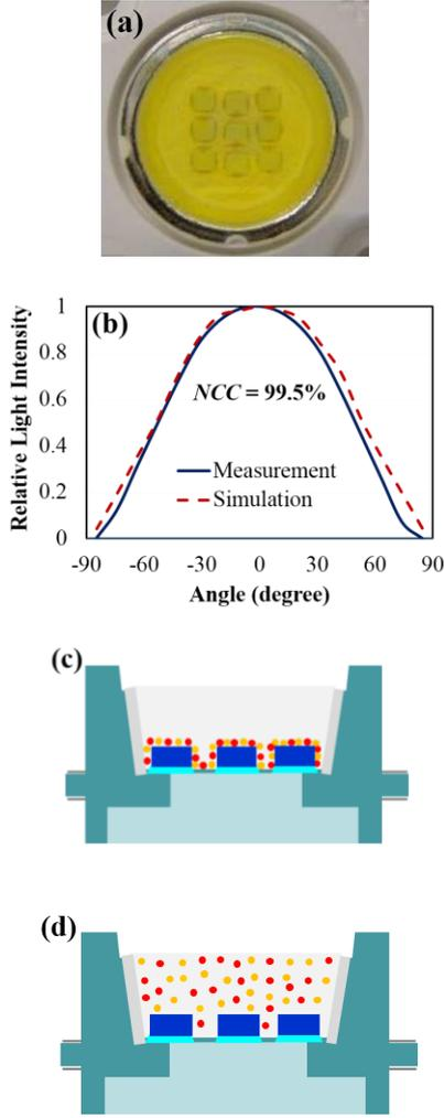
Fig. 1. Illustration of phosphor-converted WLEDs as doping  $\text{SrB}_8\text{O}_{13}:\text{Sm}^{2+}$ : (a) The actual WLEDs; (b) The calculation of normalized cross correlation (c) CPG and (d) IPG
