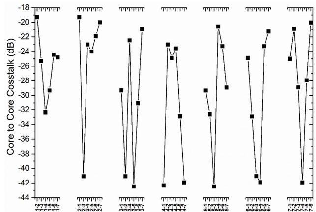
Fig. 5. Interpretation of Crosstalk for 25  $\mu\text{m}$  pitch
