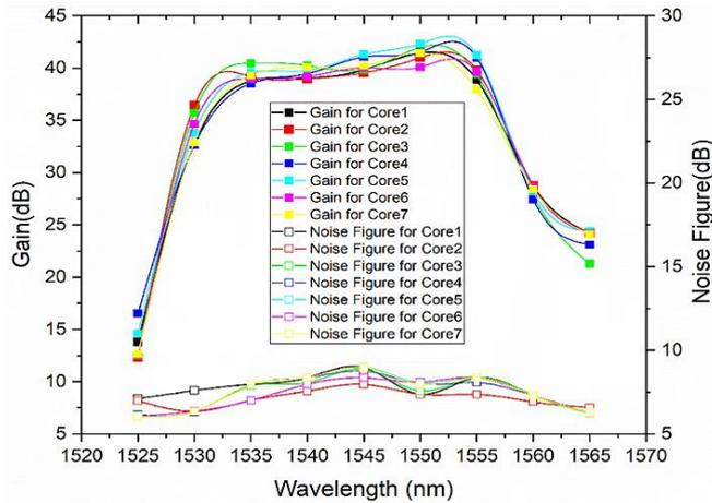
Fig. 2. Variation of Gain and Noise Figure with Wavelength for 25µm pitch (color online)
