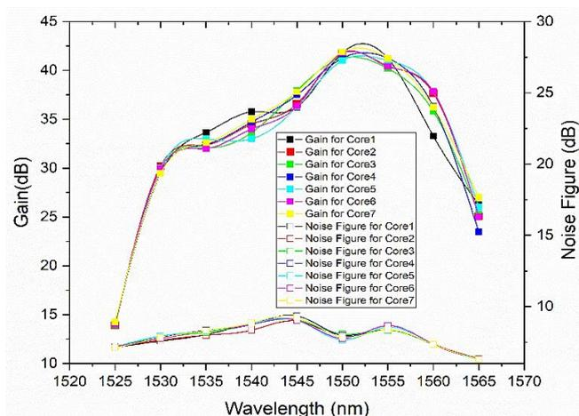
Fig. 4. Variation of Gain and Noise Figure with Wavelength for 35µm pitch (color online)
