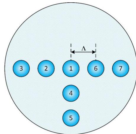
Fig. 1. Schematic of the cross-section of T-structured MC-EDFA (color online)
