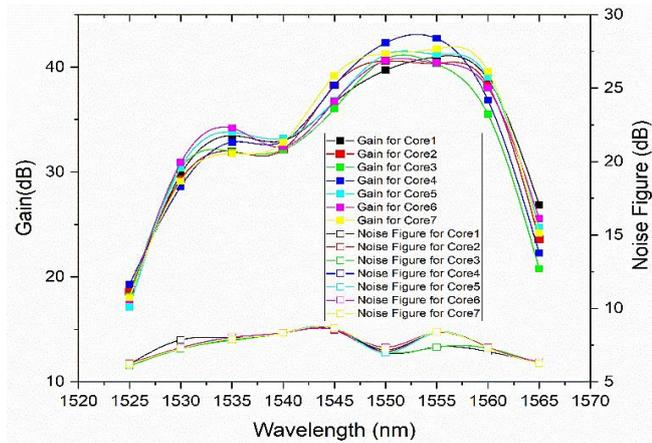
Fig. 3. Variation of Gain and Noise Figure with Wavelength for 28 µm pitch (color online)
