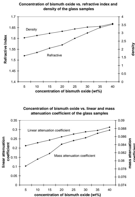
Fig. 1. Bi<sub>2</sub>O<sub>3</sub> concentration vs. density, refractive index, linear attenuation coefficient and mass attenuation coefficient of the glass samples.
