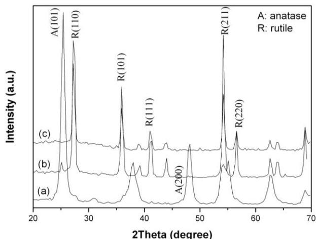
Fig. 1. XRD pattern of  $\text{TiO}_2$  nanoparticles annealed at 450, 550, and 800 °C.
