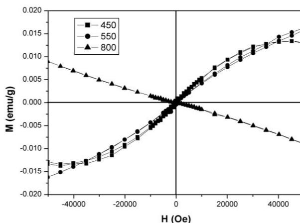
Fig. 5. M-H curves of TiO<sub>2</sub> annealed at 450, 550, and 800 °C measured at 5 K.
