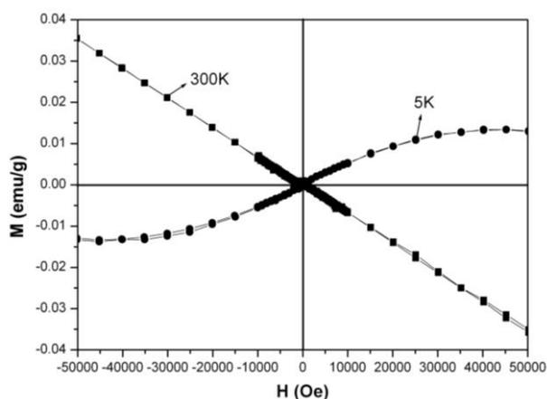
Fig. 4. M-H curves of TiO<sub>2</sub> annealed at 450 °C measured at 5 K and 300 K.
