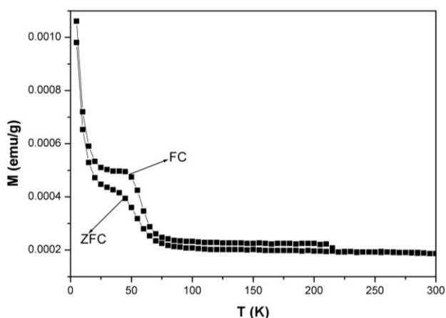
Fig. 3. ZFC and FC curves of sample annealed at 550 °C under a magnetic field of 2000 Oe.
