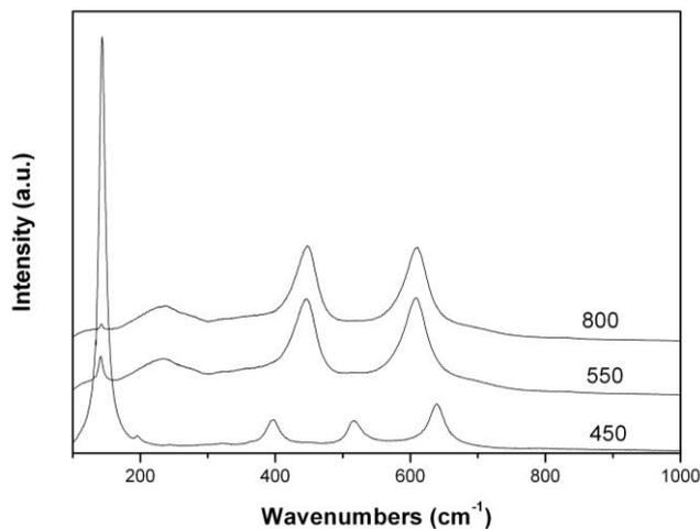
Fig. 2. Raman spectra of  $\text{TiO}_2$  nanoparticles annealed at 450, 550, and 800 °C.
