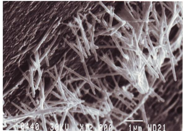
Fig. 2. SEM micrograph of 100 nm silver iodide nanowires.
