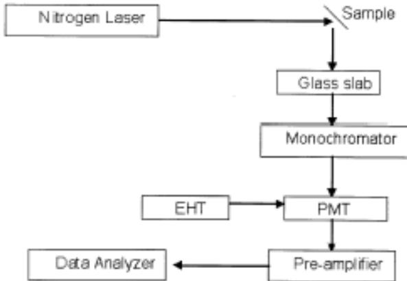
Fig. 1. Photoluminescence setup.
