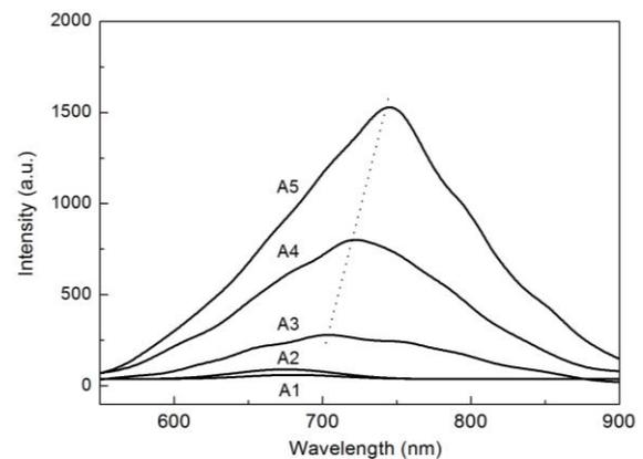
Fig. 4. PL spectra of A serial specimen (without Al-doping and annealed at 400-800 °C).
