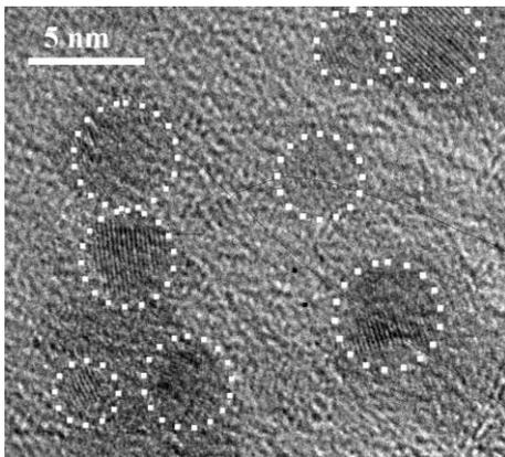
Fig. 2. HR-TEM image of sample B2 (Al-doping at a dose of  $4 \times 10^{14}$  cm<sup>-2</sup> and annealed at 500 °C).
