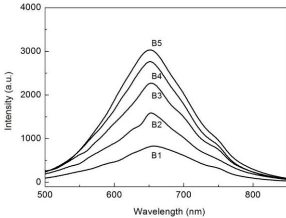
Fig. 5. PL spectra of B serial specimen (with Al-doping and annealed at 400-800 °C).
