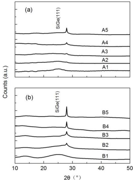
Fig. 1. XRD diffraction spectra of specimen A (a) and B (b) serial.
