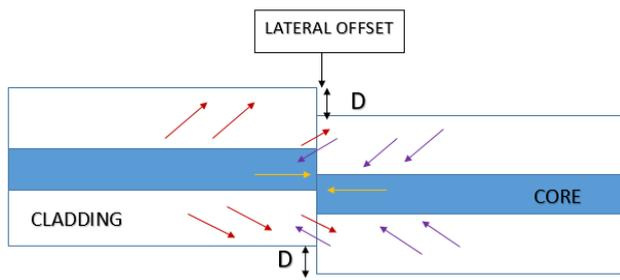
Fig. 1. Schematic Diagram of Lateral Offset
