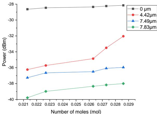
Fig. 7. Graph of output power (dBm) vs the number of mole (mol) of coconut-palm oil mixture for various lateral offset distance (color online)
