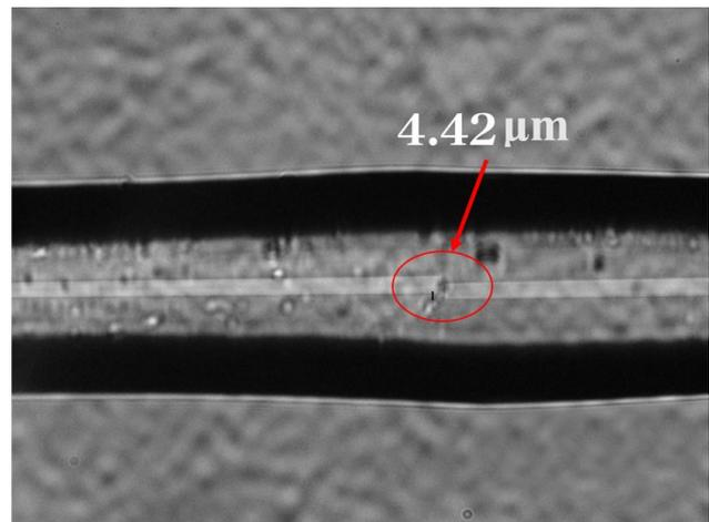
Fig. 3. Recorded Image from Image Analyzer for  $4.42\mu\text{m}$  lateral offset
