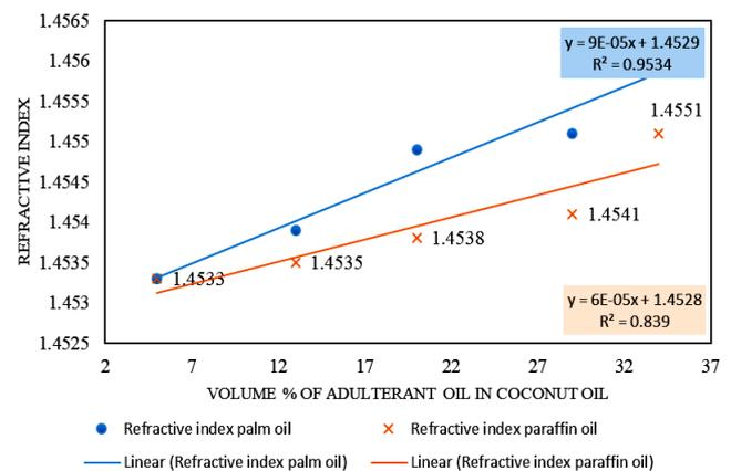
Fig. 6. Refractive index of the volume percentage of palm oil and paraffin oil in coconut oil (color online)
