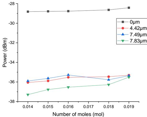
Fig. 8 Graph of output power (dBm) versus the number of moles (mol) coconut oil with paraffin oil with all distance ( $\mu\text{m}$ ) by using MMF-MMF (color online)
