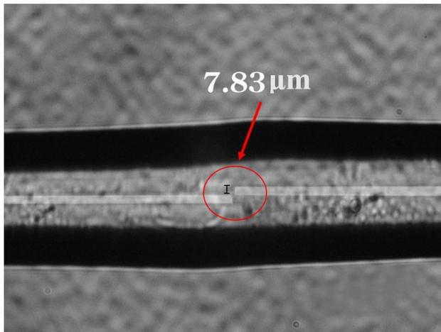
Fig. 5. Recorded image from image analyzer for 7.83  $\mu\text{m}$  lateral offset
