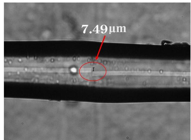
Fig. 4. Recorded Image from Image Analyzer for  $7.49\mu\text{m}$  lateral offset
