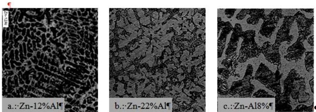
Fig. 3. Structural aspects of Zn-Al alloys: (a) Zn-12%Al cast (X500); (b) Zn-22%Al cast (X500); (c) Zn-8%Al heat treated (X1000).
