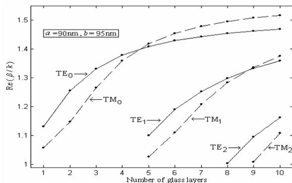
Fig. 5. The real part of the exact effective propagation constants as a function of number of glass layers for the modes  $TE_0$ ,  $TM_0$ ,  $TE_1$ ,  $TM_1$ ,  $TE_2$  and  $TM_2$  of the multiple superconducting quantum well structure ( $a = 90\text{nm}$ ,  $b = 95\text{nm}$ ).
