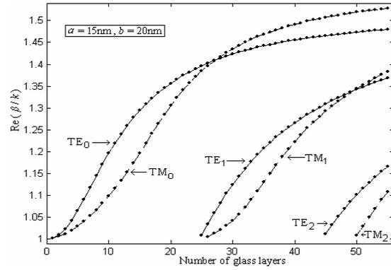
Fig. 3. The real part of the exact effective propagation constants as a function of number of glass layers for the modes  $TE_0$ ,  $TM_0$ ,  $TE_1$ ,  $TM_1$ ,  $TE_2$  and  $TM_2$  of the multiple superconducting quantum well structure ( $a = 15\text{nm}$ ,  $b = 20\text{nm}$ ).
