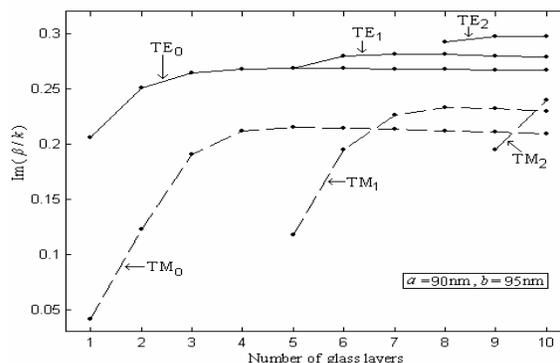
Fig. 6. The imaginary part of the exact effective propagation constants as a function of number of glass layers for the modes  $TE_0$ ,  $TM_0$ ,  $TE_1$ ,  $TM_1$ ,  $TE_2$  and  $TM_2$  of the multiple superconducting quantum well structure ( $a = 90\text{nm}$ ,  $b = 95\text{nm}$ ).
