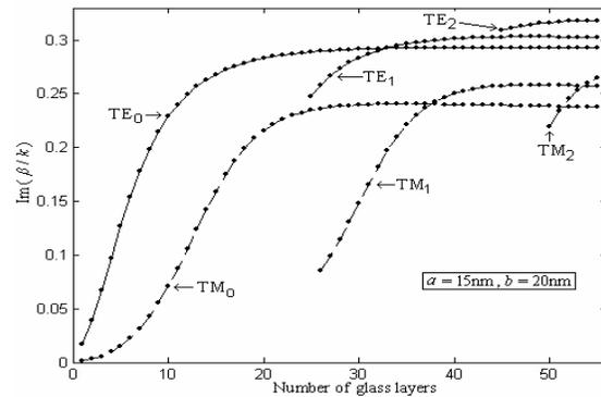
Fig. 4. The imaginary part of the exact effective propagation constants as a function of number of glass layers for the modes  $TE_0$ ,  $TM_0$ ,  $TE_1$ ,  $TM_1$ ,  $TE_2$  and  $TM_2$
