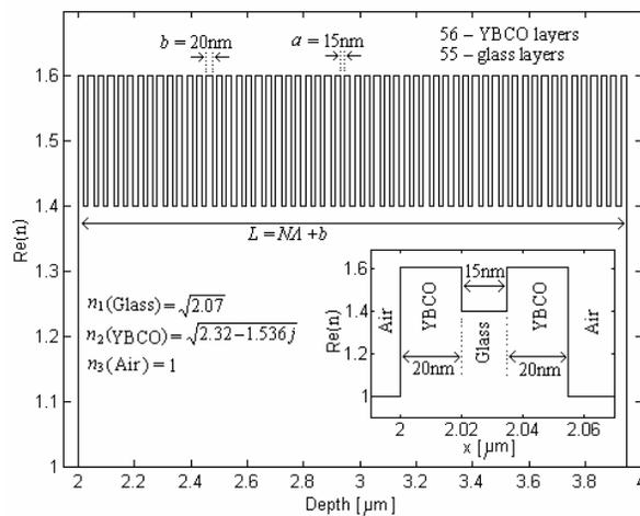
Fig. 1. The real part of the refractive index profile for a multiple superconducting well structure. The inset is a structure with a single glass layer.
