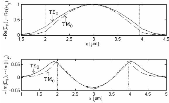
Fig. 2. The real part and imaginary parts of the fundamental field profiles ( $-E_y$ ,  $-H_y$ ) of a multiple superconducting well waveguide with 55 glass layers ( $a = 15\text{nm}$ ,  $b = 20\text{nm}$ ) as a function of the depth distance.
