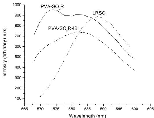
Fig. 3. Fluorescence spectra of LRSC and rhodamine derivatives ( $PVA-SO_2R$ ,  $PVA-SO_2R-IB$ ) in buffer solution ( $pH = 7.2$ ).
