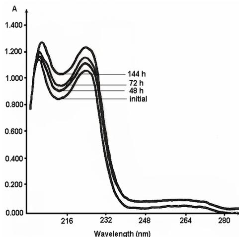
Fig. 4. Variation in time of ibuprofen absorbance in the UV spectrum (221 nm) in buffer solution ( $pH = 7.2$ ).
