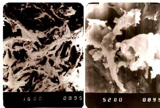
Fig. 2. SEM images of PVA-SO<sub>2</sub>R-IB hybrid composite at different resolutions: (a) X 1600, (b) X 5200.
