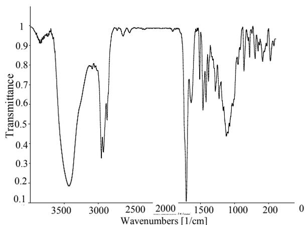
Fig. 1. FTIR spectrum of PVA-SO<sub>2</sub>R-IB hybrid composite.
