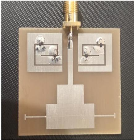
Fig. 15. Fabricated prototype of the proposed antenna
