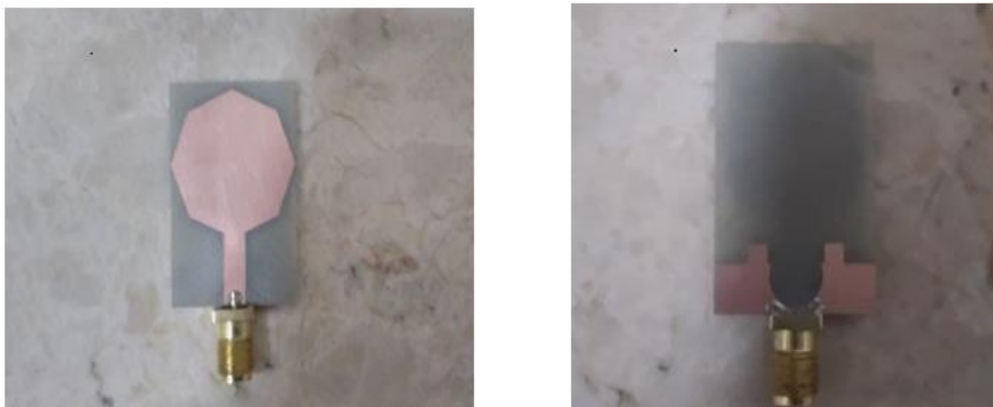
Fig. 9. Snapshots of the projected monopole antenna in terms of front and back views
