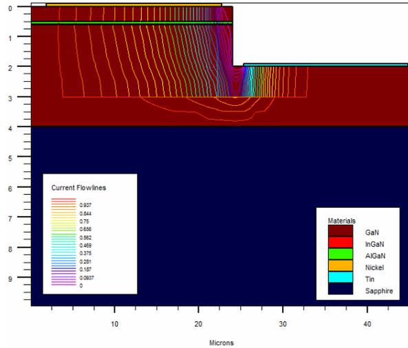
Fig. 6. Current flow-lines in conventional III-nitride LED with delta doping.
