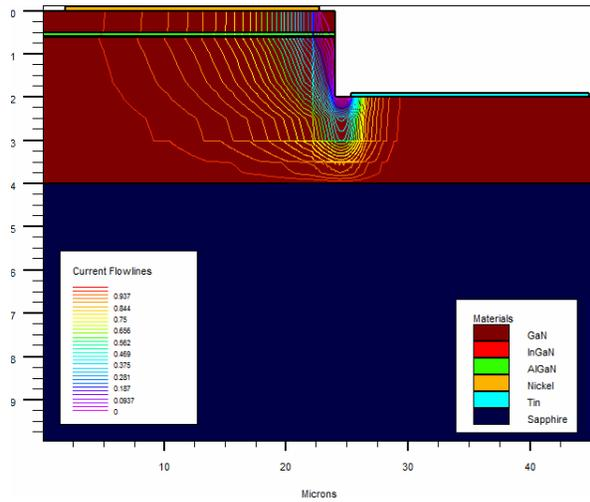
Fig.2. Current flow-lines in Conventional III-nitride LED.
