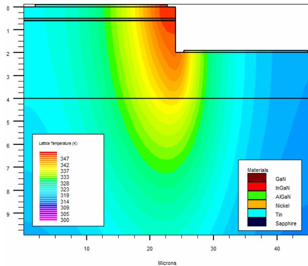
Fig.3. Temperature in Conventional III-nitride LED, forward bias at 7V.
