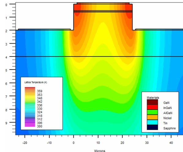
Fig.5. Temperature in multi-finger III-nitride LED, forward bias at 7V.
