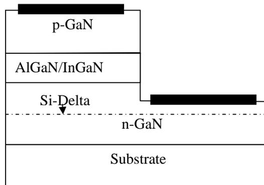
Fig.1. Schematic of III-nitride LED.
