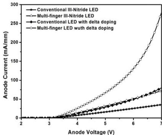
Fig.8. V-I characteristics of III-nitride devices.
