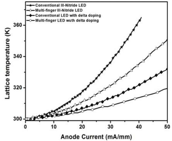
Fig. 9. Lattice temperature vs. Anode current of III-nitride devices.
