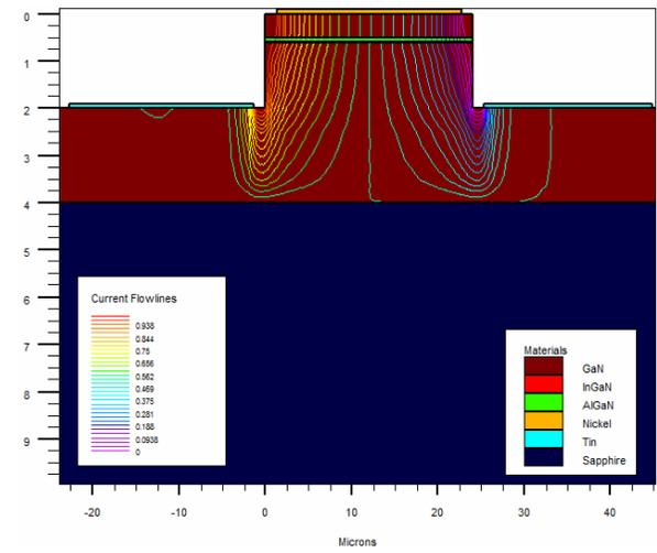
Fig.4. Current flow-lines in Multi-finger III-nitride LED.
