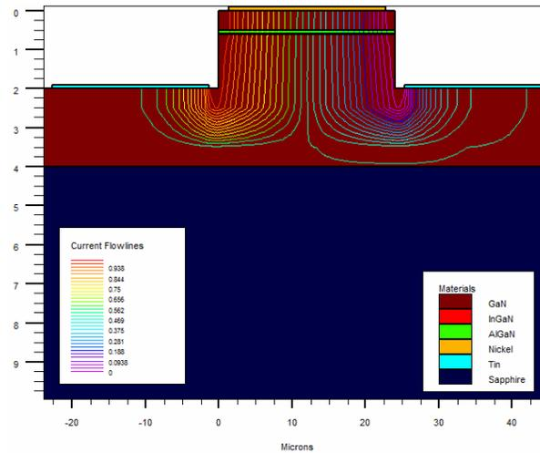
Fig.7. Current flow-lines in multi-finger III-nitride LED.
