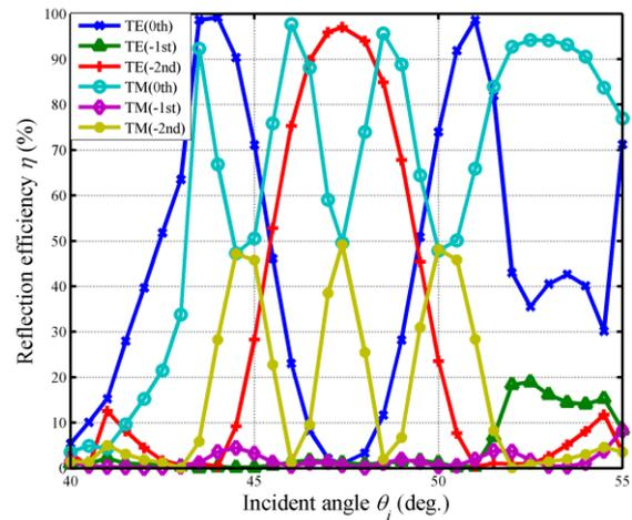
Fig. 5. (Color online) Reflection efficiency versus incident angle for a wavelength of 800 nm with the same optimized grating profile parameters as Fig. 4.
