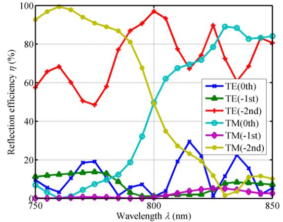
Fig. 4. (Color online) Reflection efficiency versus incident wavelength under second Bragg angle mounting, duty cycle  $f = 0.5$ , period  $d = 748 \text{ nm}$  and depth  $h = 2.73 \mu\text{m}$ .
