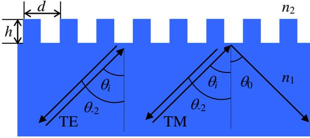
Fig. 1. (Color online) Schematic of a dual-function grating element under TIR and second Bragg angle mounting ( $n_1$  and  $n_2$  refractive indices of fused silica and air, respectively,  $d$  period,  $h$  depth,  $\theta_i$  incident angle,  $\theta_0$  and  $\theta_2$  diffraction angles of the 0<sup>th</sup> and -2nd reflection orders in fused silica, respectively).
