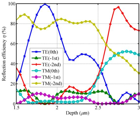
Fig. 3. (Color online) Reflection efficiency of a TIR grating versus depth with the optimized period of 748 nm and duty cycle of 0.5 for the wavelength of 800 nm under second Bragg angle mounting.
