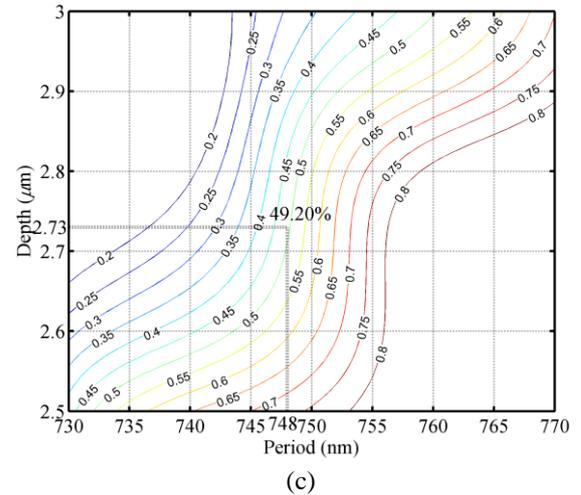
Fig. 2. (Color online) The Contour of the efficiency of a TIR grating versus grating period and depth with the duty cycle of 0.5 for the wavelength of 800 nm under second Bragg angle mounting: (a) TE polarization in the -2nd order, (b) TM polarization in the 0th order, (c) TM polarization in the -2nd order.
