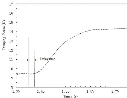
Fig. 5. Method to find the delay time
