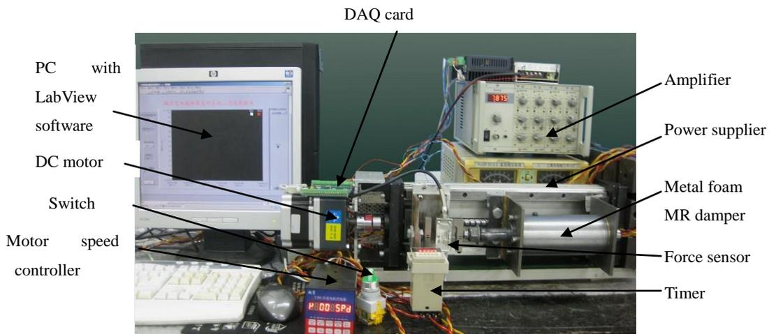
Fig. 3. Test rig of foam MR damper
