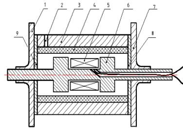
1,7 End cap of cylinder Piston rod; 2 Gap; 3 Cylinder; 4 Porous foam nickel; 5 Coil; 6 Piston; 8,9 Bronze
