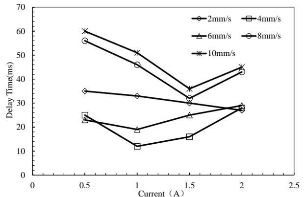
Fig. 6. Changes of delay time of porous foam metal MR damper as a function of current at different shear velocity
