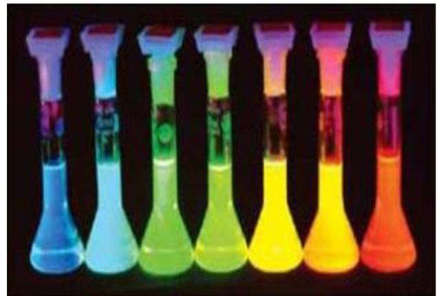
Fig. 5. Fluorescence in different-sized CdSe quantum-dots [11].
