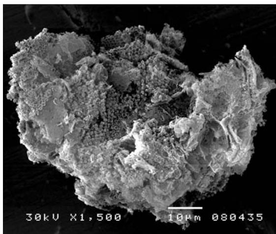
Fig. 4. SEM micrograph of powders obtained after 4 h at 1450 °C.
