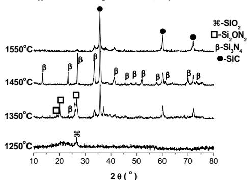
Fig. 2. Comparative XRD patterns after different heat treatments and constant heating time, 4 h of mixture diatomaceous earth-commercial sugar.
