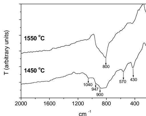
Fig. 3. IR comparative transmission spectra of the mixture after different heat treatments and constant heating time, 4 h of mixture diatomaceous earth-sugar.
