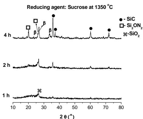
Fig. 1. XRD patterns after constant heat treatments and different heating time, SiO<sub>2</sub>-cristoballite.
