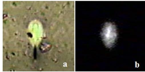
Fig. 1. (a) The optical microscopic image of single mode waveguide structure with 50x magnification under white light illumination and (b) its corresponding near field image at 1550 nm wavelength.
