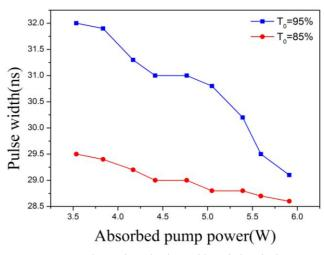
Fig. 7. Relationship of pulse width and absorbed pump power (color online)
