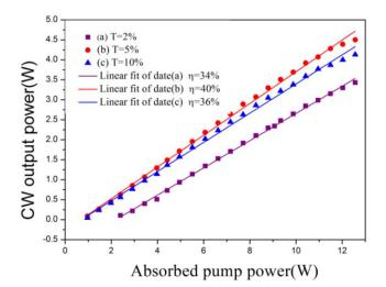
Fig. 2. Relationship of CW output power and absorbed pump power with output mirrors of varies transmission (color online)
