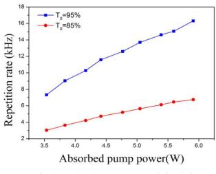
Fig. 6. Relationship of repetition rate and absorbed pump power (color online)
