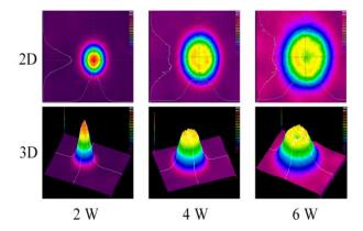
Fig. 3. Beam profiles of CW Nd:GGG laser at various absorbed pump power (color online)
