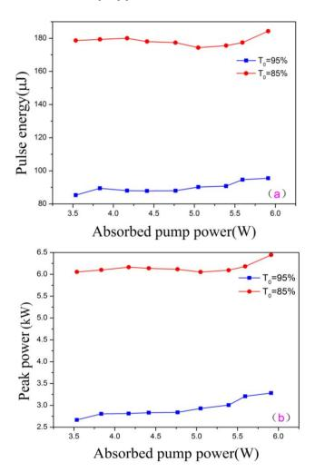
Fig. 8. Relationship of pulse performance and absorbed pump power: (a) pulse energy; (b) pulse peak power (color online)
