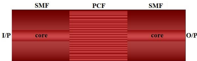
Fig. 3. Proposed design of the sensor. I/P is the input where the signal is fed into the sensor and O/P is the output where the signal is analyzed
