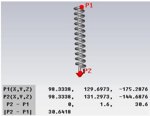
Fig. 1. Helix antenna used in the simulation.
