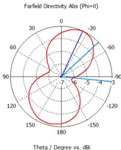
Fig. 2. Helix antenna radiation pattern.
