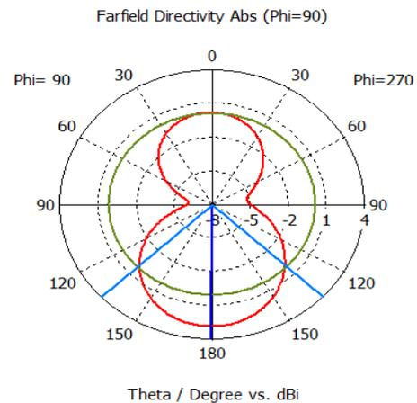
Fig. 4. PIFA antenna radiation pattern.
