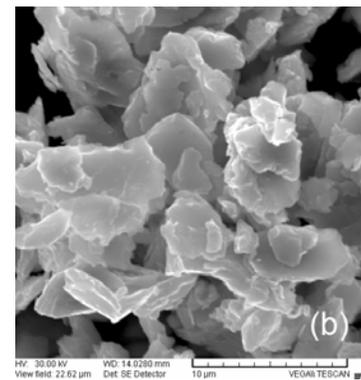
Fig. 4. SEM images for NANOPERM powders ball-milled for 90 h, at different magnifications.
