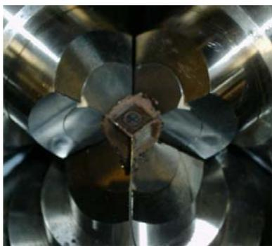
Fig. 3. Relative position of anvils and sample holder.
