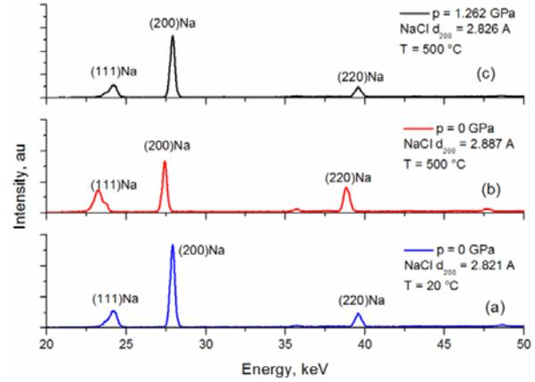
Fig. 5. Diffraction pattern of NaCl at different temperatures and applied pressures.
