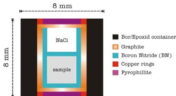
Fig. 2. Sample holder construction scheme.
