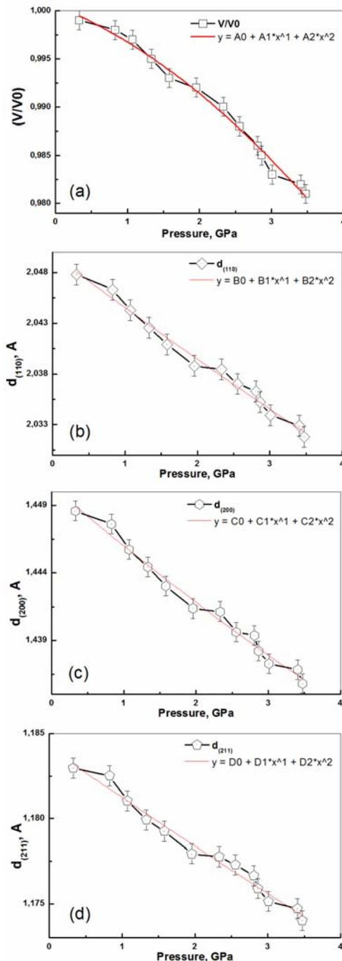
Fig. 6. Pressure influence upon crystalline cell volume (a) and interplanar distances  $d_{(110)}$  (b);  $d_{(200)}$  (c) and  $d_{(211)}$  (d).
