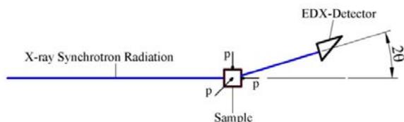
Fig. 1. Schematic representation of measurement method.
