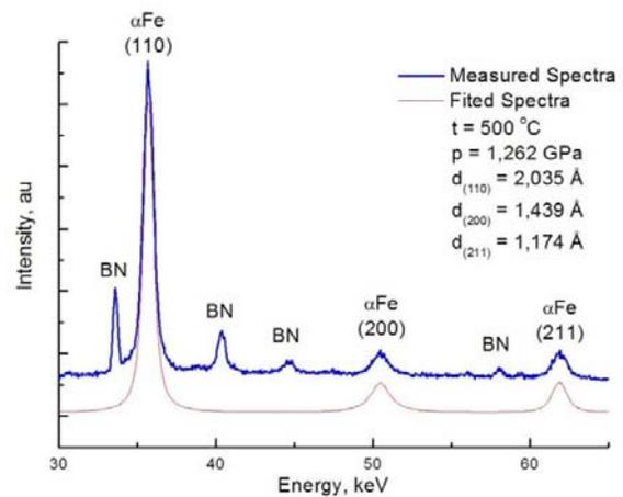
Fig. 6. Diffraction pattern of NANOPERM powders at  $p = 1.262$  GPa and  $t = 500^\circ\text{C}$ .
