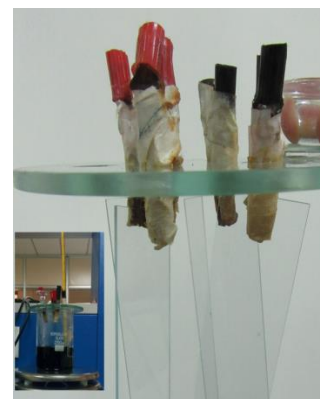
Fig. 1. Substrate fixing setup used for the deposition
