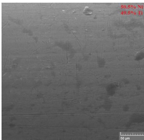
Fig. 1. SEM microscopy of initial NiTi state surface, 250x.
