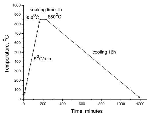
Fig. 1. Thermal treatment diagram for chemical activation of MCMB.
