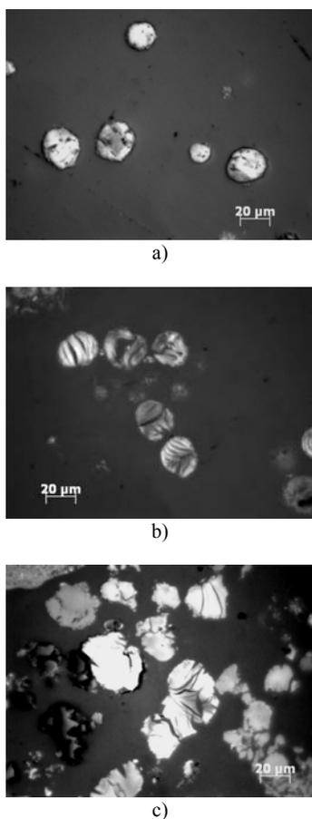
Fig. 2. Optical micrographs of: a) MCMB, b) activated MCMB with NaOH, c) activated MCMB with KOH.
