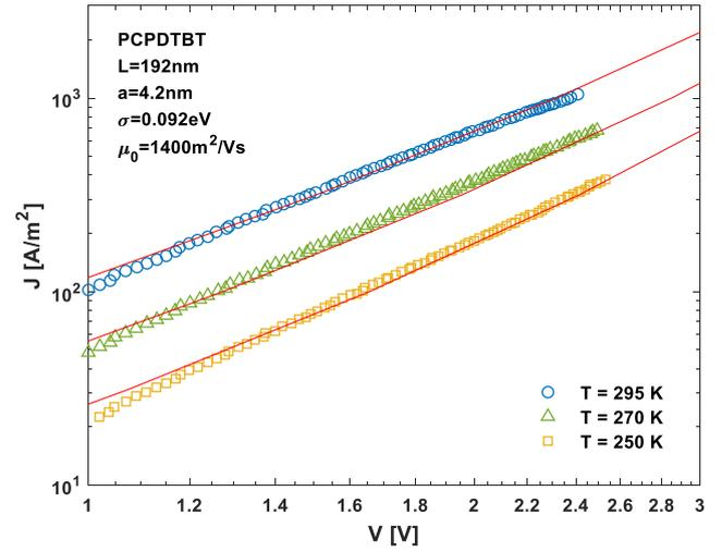
Fig. 1. Temperature dependent  $J - V$  characteristics of PCPDTBT hole-only device with a layer thickness of 192 nm. Symbols are the experimental data from Ref. [24]. Lines are the numerically calculated results based on the IEGDM (color online)
