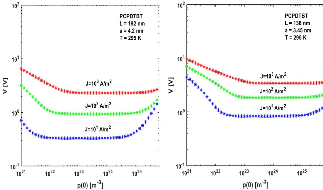
Fig. 3. Theoretical results of voltage versus the boundary carrier density of PCPDTBT hole-only (Left) and electron-only (Right) devices at room temperature. Different lines correspond to different current density values (color online)
