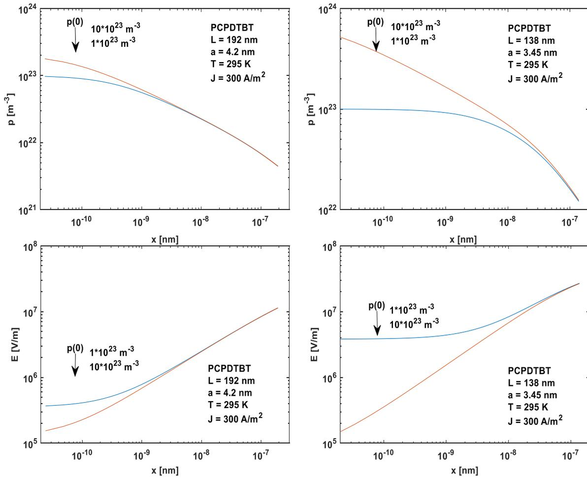
Fig. 4. Numerically calculated distribution of the charge carrier density  $p$  and electric field  $E$  as a function of the distance  $x$  in PCPDTBT hole-only (Left) and electron-only (Right) devices at room temperature (color online)
