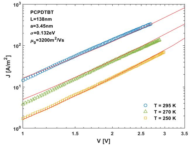
Fig. 2. Temperature dependent  $J - V$  characteristics of PCPDTBT electron-only device with a layer thickness of 138 nm. Symbols are the experimental data from Ref. [24]. Lines are the numerically calculated results based on the IEGDM (color online)
