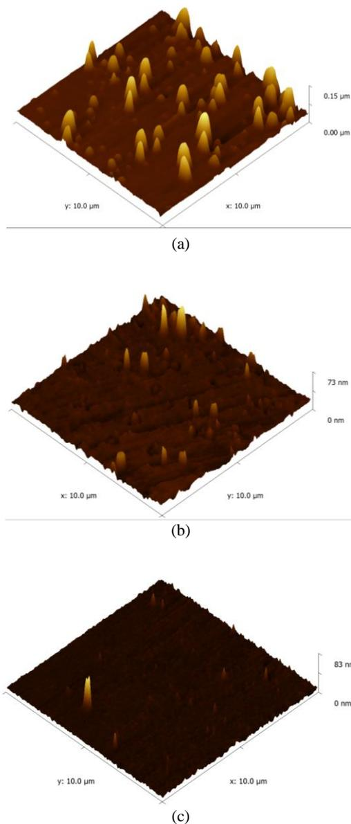
Fig. 1. 3D AFM images of the deposited thin films.
