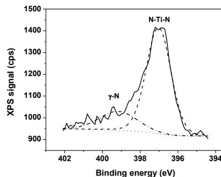
Fig. 5. The deconvolution of the N 1*s* high resolution spectrum of the sample S2.
