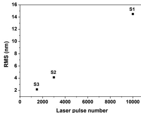
Fig. 2. The dependence of the RMS on the laser pulses number.
