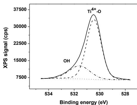
Fig. 4. The deconvolution of the O 1*s* high resolution spectrum of the sample S2.
