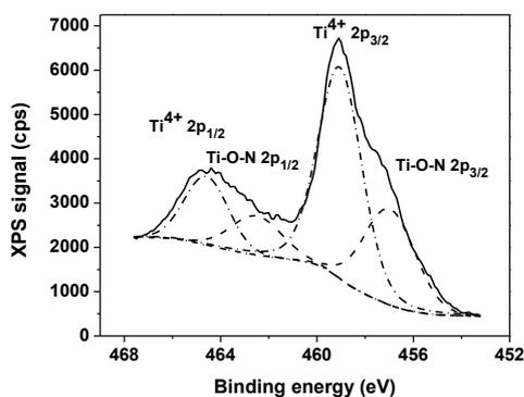
Fig. 3. The deconvolution of the Ti 2*p* high resolution spectrum of the sample S2.
