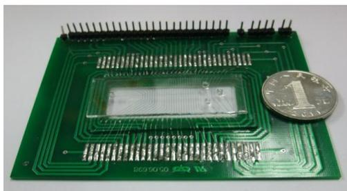
Fig. 7. Successful bonding chip attached the PCB board.
