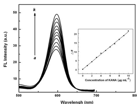
Fig. 5. Fluorescence emission spectra of CdTe/CdSe QDs in the absence and presence of different concentration of KANA (0.0, 1.0, 2.0, 3.0, 4.0, 5.0, 6.0, 7.0, 8.0, 9.0 and 10.0  $\mu\text{g mL}^{-1}$  from a to k). Inset: Plot of fluorescence enhancement [ $\Delta F$ ] of CdTe/CdSe QDs at emission peak versus [KANA].
