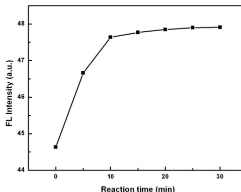
Fig. 4. Effect of reaction time on the fluorescence intensity of CdTe/CdSe QDs.
