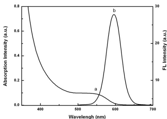
Fig. 1. UV-vis absorption (a) and fluorescence spectra (b) of CdTe/CdSe QDs.
