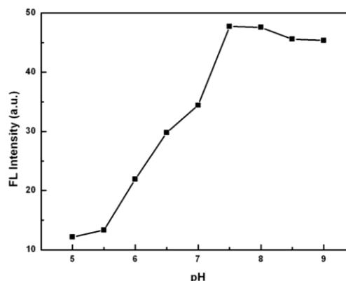
Fig. 3. Effect of pH on the fluorescence intensity of CdTe/CdSe QDs.
