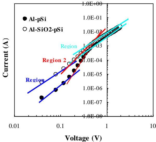
Fig. 5. The forward bias  $\log(I)$ - $\log(V)$  plot of the Al/p-Si and Al/SiO<sub>2</sub>/p-Si Schottky diodes.
