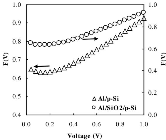
Fig. 4.  $F(V)$  -  $V$  graph of the Al/p-Si and Al/SiO<sub>2</sub>/p-Si Schottky diodes.
