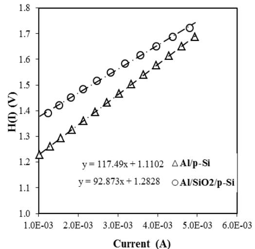
Fig. 3. The experimental  $H(I)$ – $I$  plot for the Al/p-Si and Al/SiO<sub>2</sub>/p-Si Schottky diodes.
