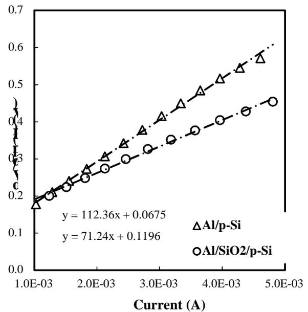
Fig. 2. The experimental  $dV/d(\ln I)$ – $I$  plot for the Al/p-Si and Al/SiO<sub>2</sub>/p-Si Schottky diodes.
