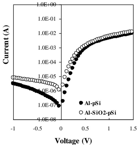
Fig. 1. The plots of the current–voltage ( $I$ – $V$ ) characteristics for Al/p-Si and Al/SiO<sub>2</sub>/p-Si Schottky diodes.
