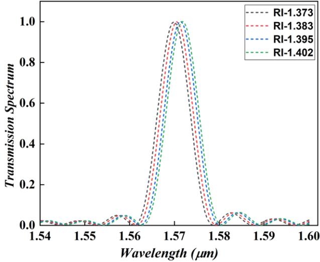
Fig. 6. Transmission spectrum of refractive index ranging from 1.373 to 1.402 (color online)
