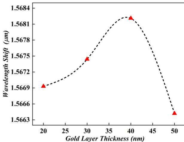
Fig. 4. Wavelength shift vs gold layer thickness (color online)
