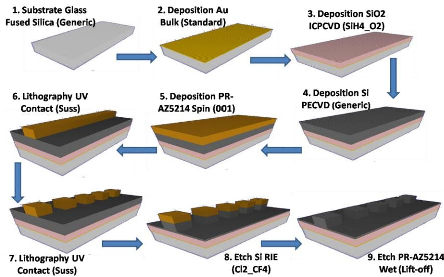
Fig. 7. Process flow steps for the proposed SOI waveguide based sensor (color online)
