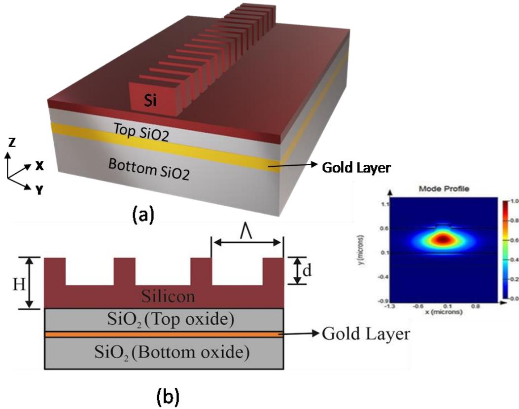
Fig. 1. (a) Rib waveguide with gratings is depicted schematically supporting single mode. (b) Side view of the device (color online)
