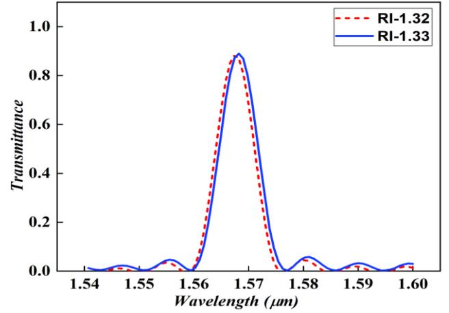
Fig. 2. Transmittance plot with RI 1.32 and 1.33 (color online)
