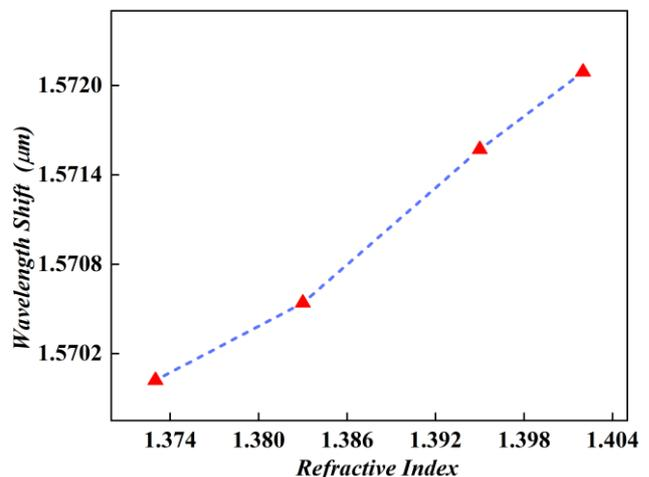
Fig. 5. Wavelength shift vs refractive index change (color online)
