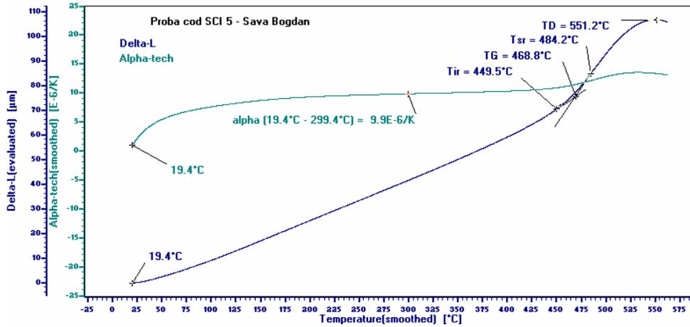
Fig. 2. The thermal expansion curve for the sample SCI5.
