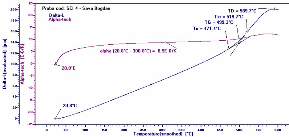
Fig. 1. The thermal expansion curve for the sample SCI4.
