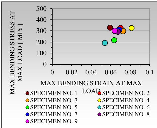
Fig. 5. Maximum bending stress at maximum load distribution of five layers Heliopol/Stratimat 300.
