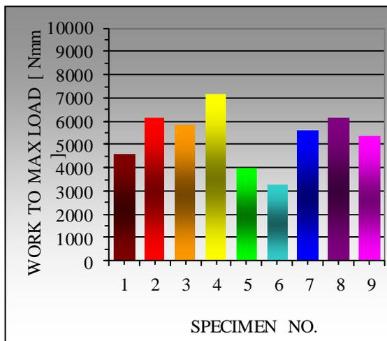
Fig. 6. Work to maximum load distribution of five layers Heliopol/Stratimat300 composite laminate.
