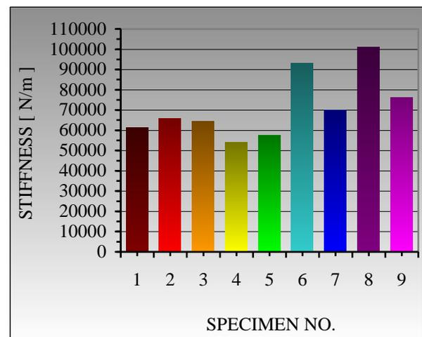
Fig. 2. Stiffness distribution of five layers Heliopol/Stratimat300 composite laminate.
