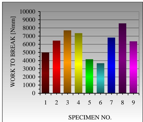
Fig. 9. Work to break distribution of five layers Heliopol/Stratimat300 composite laminate.
