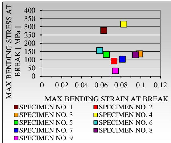
Fig. 8. Maximum bending stress at break distribution of five layers Heliopol/Stratimat300.
