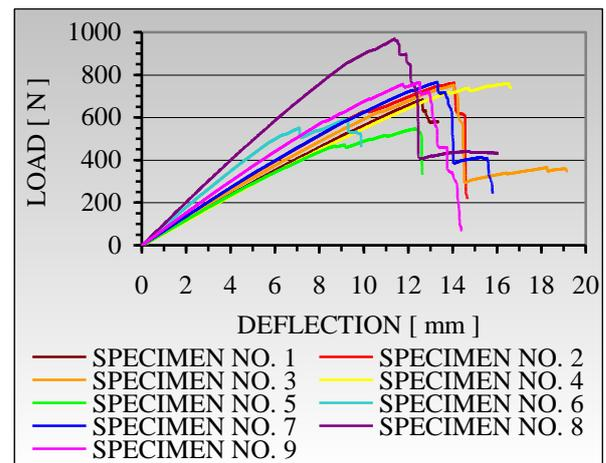
Fig. 1. Load-Deflection distribution of five layers Heliopol/Stratimat300 composite laminate.
