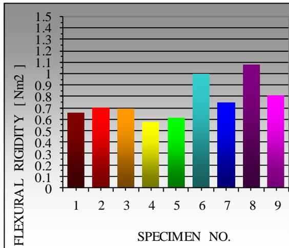
Fig. 4. Flexural rigidity distribution of five layers Heliopol/Stratimat300 composite laminate.
