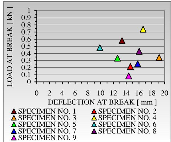
Fig. 7. Load-deflection at break distribution of five layers Heliopol/Stratimat300 composite laminate.
