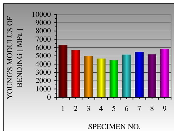
Fig. 3. Young's modulus of bending distribution of five layers Heliopol/Stratimat300 composite laminate.
