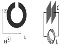
Fig. 1. SRR inclusion and lumped circuit.
