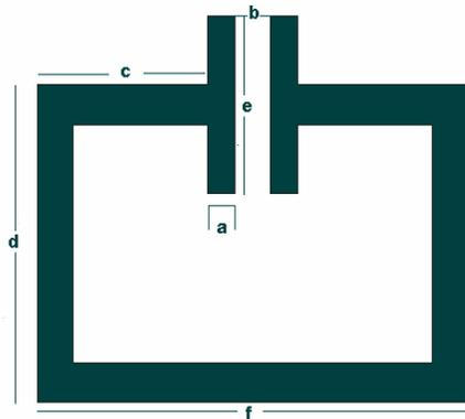
Fig. 2. ICSRRs inclusion and dimension:  $a = 0.19 \text{ mm}$ ;  $b = 0.38 \text{ mm}$ ;  $c = 1.15 \text{ mm}$ ;  $d = 2.03 \text{ mm}$ ;  $e = 1.15 \text{ mm}$ ;  $f = 3.05 \text{ mm}$ .
