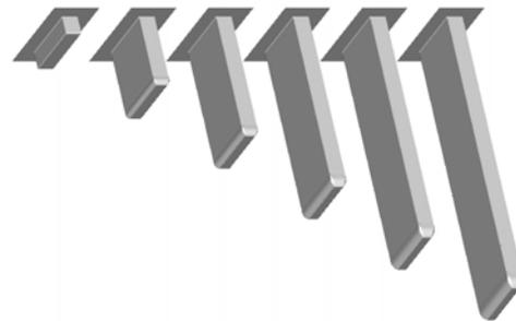
Fig. 2. Anisotropic etching - Feature profiles for  $R = R_0 \cos \theta$  at six equidistant (reduced) etching time moments.
