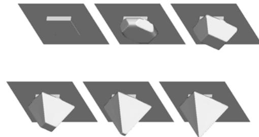
Fig. 3. Etching through a square mask in  $\{100\}$  plane aligned to  $\langle 100 \rangle$  directions. Profiles at six equidistant (reduced) time moments.
