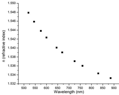
Fig. 3. The variation of refractive index with the wavelength.
