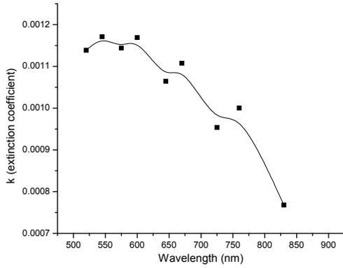
Fig. 2. The variation of extinction coefficient with the wavelength.
