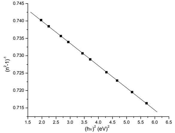
Fig. 4. Plot of  $(n^2 - 1)^{-1}$  vs.  $(h\nu)^2 (eV)^2$  for polystyrene thin films.
