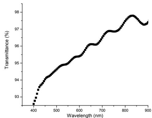
Fig. 1. Transmission spectrum of polystyrene thin film.
