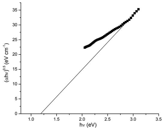
Fig. 5. Plot of  $(ahv)^{0.5}$  vs. photon energy for polystyrene thin films.
