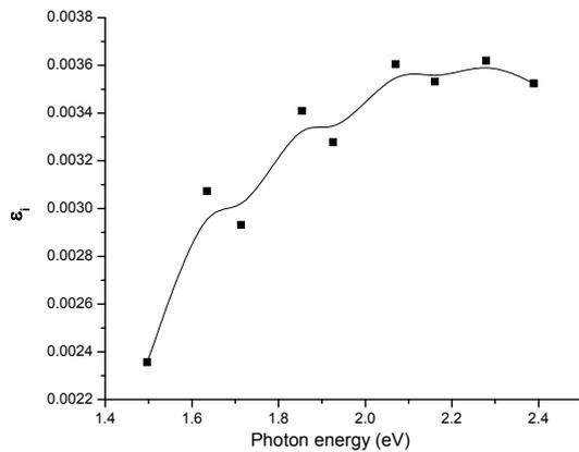
Fig. 6. Plot of  $\epsilon_i$  vs. photon energy for polystyrene thin film.
