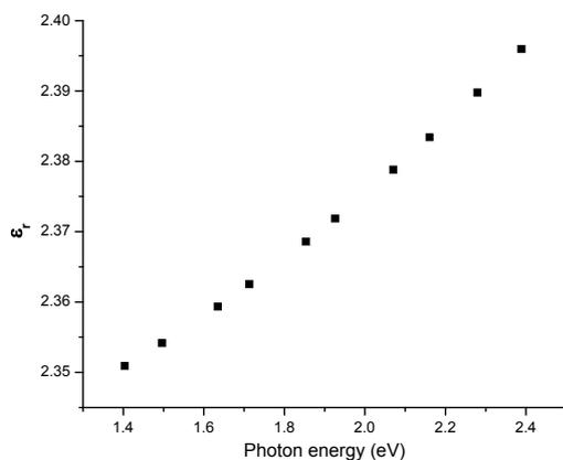
Fig. 7. Plot of  $\epsilon_r$  vs. photon energy for polystyrene thin film.
