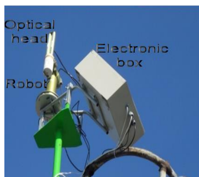
Fig. 1. Main components of the sun photometer from Timisoara.
