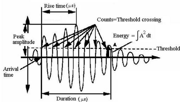
Fig. 3. AE Signal Characteristic Features [12].
