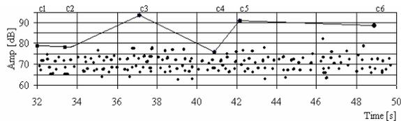
Fig. 8. AE signal corresponding to the scratch test from fig. 7.
