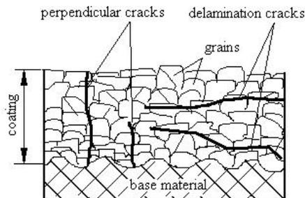
Fig.1 . Types of cracks into a coating [8].
