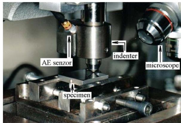
Fig. 5. LSRH-Revêtest scratch tester with the acoustic sensor on the indentation shaft. The micrograph of a scratching test.
