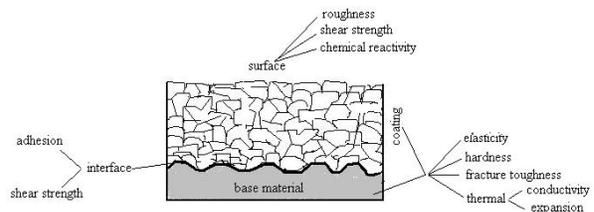
Fig. 2. Some properties of different zones of the surface, coating, interface and substrate.
