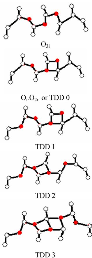
Fig. 2. Structural models of  $O_{3i}$ , TDD0, TDD1, TDD2, TDD3 correspond to equations given above. Positions of the atoms are not to the scale. White circles are for Si atoms and red circles are oxygen atoms.
