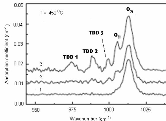
Fig. 1. Fragment of absorption spectra at  $450 \text{ }^\circ\text{C}$  for CZ-Si.
