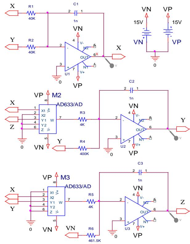
Fig. 3. Electronics circuit model of the BSCS.
