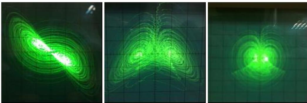
Fig. 5. Oscilloscope outputs of the realized Burke-Shaw chaotic oscillator. (a) x-y signals phase portrait (b) x-z signals phase portrait (c) y-z signals phase portrait.
