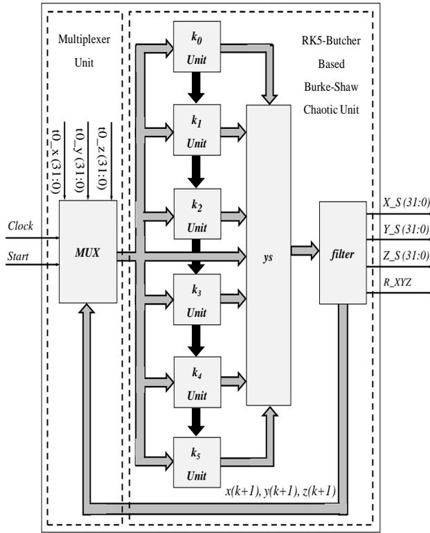
Fig. 6. Block diagram of Burke-Shaw chaotic oscillator unit.
