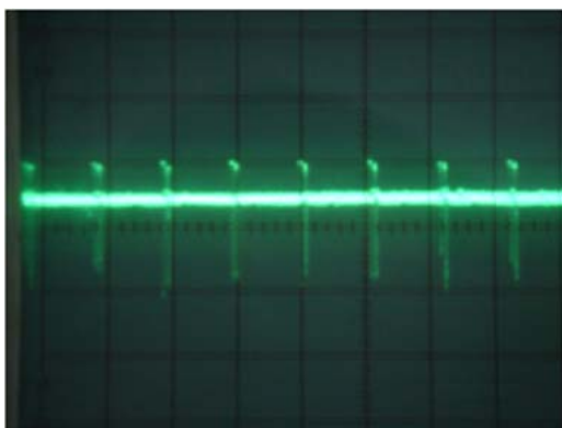
Fig. 2. Pulse train of the acousto-optic Q-switched \text{Yb}^{3+} -doped all-fiber laser.
