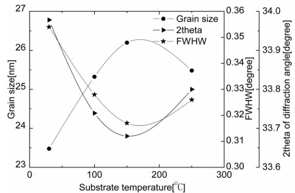
Fig. 2. Grain size, FWHM and 2theta of diffraction angle as a function of substrate temperature.
