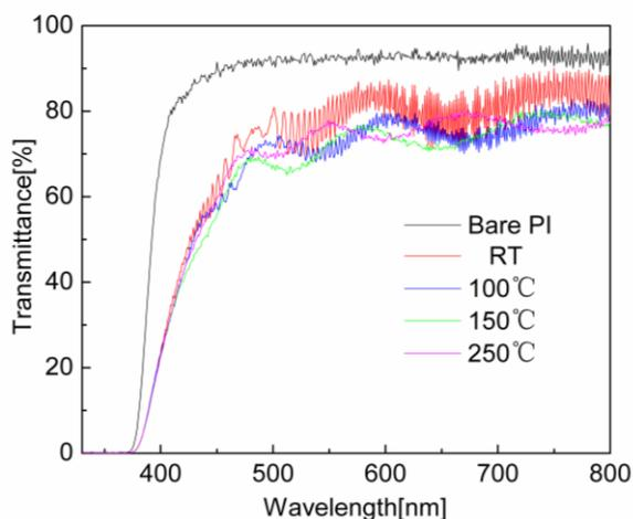
Fig. 4. Optical property of bare PI and AZO films deposited on PI substrate.
