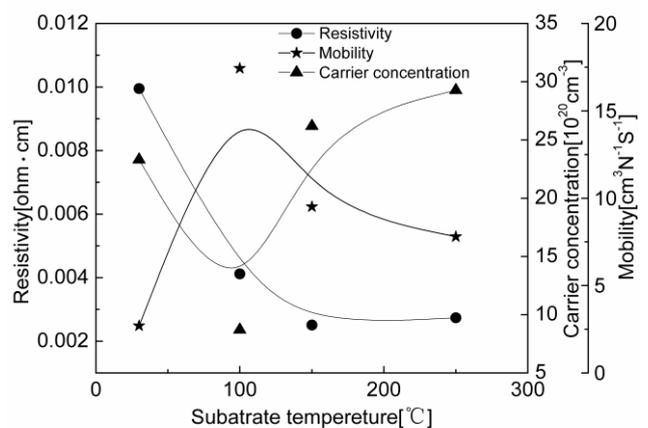
Fig. 3. Resistivity, mobility and carrier concentration as a function of substrate temperature.
