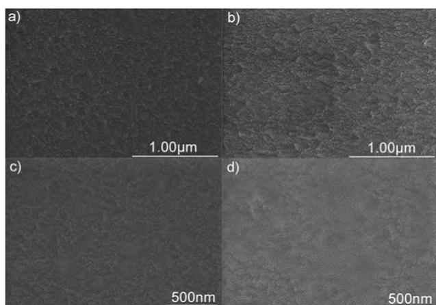
Fig. 5. SEM micrographs of AZO films deposited on PI substrate at different temperature: (a) room temperature, (b) 100 °C (c) 150 °C (d) 250 °C
