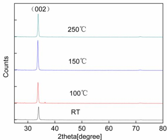
Fig. 1. XRD diffraction patterns of the AZO films deposited at sputtering power of 60W and working pressure of 1.0Pa on the polyimide substrate with different substrate temperatures (from RT to 250 °C).
