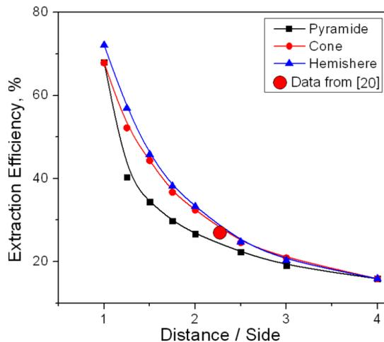
Fig. 5. Extraction efficiency vs. DD parameter for different 3D textures.
