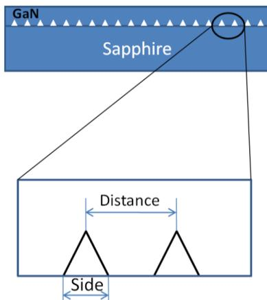
Fig. 2. Air prism embedded reflector.
