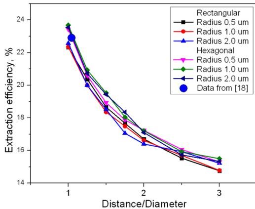
Fig. 1. Extraction efficiency vs. DD parameter for different sizes of hemisphere and packaging.
