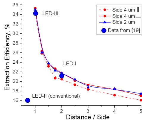
Fig. 3. Extraction efficiency vs. DD parameter for different prism heights.
