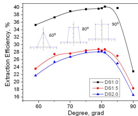
Fig. 4. Extraction efficiency vs. base angle for different Distance/Side values.
