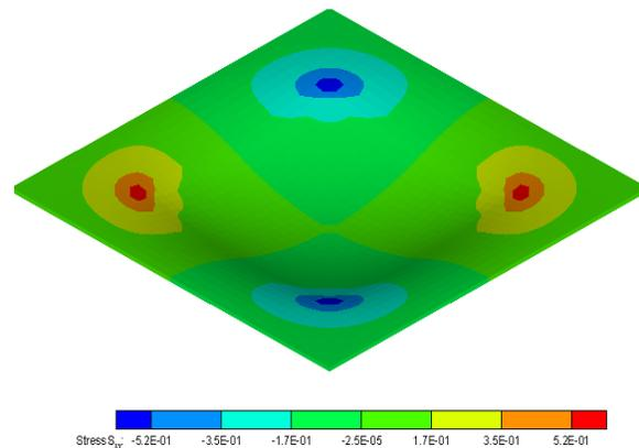
Fig. 4. The mechanical stress in MPa, in the Si-membrane, actuated by the piezoelectric layer biased at 5V.
