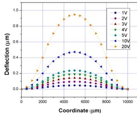
Fig. 2. Graph of the membrane deflection versus horizontal coordinate for positive  $V_{F-B}$  from 1V to 20V.
