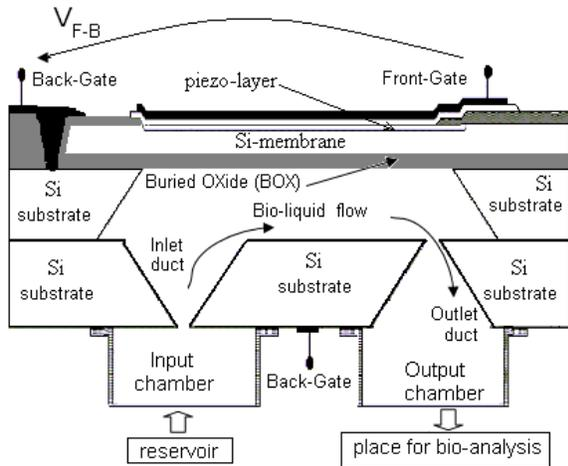
Fig. 1. The proposed SOI-MEMS structure.
